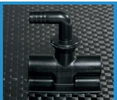
The **Blade Runner® Connector** has been developed specially for the resin feed line **Blade Runner®**. With this connector, inlet points can be set easily and safely. The **Connector** is placed on the resin line. The matching connection tap is then inserted from above. Two different connection taps are available: One vertical and one angled. Appropriately assembled sealing rings are placed between the connector and the connecting tap. These sealing rings ensure an airtight connection.
