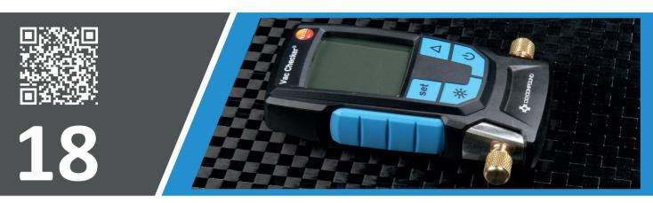
Digital vacuum gauge **Vac Checker**® from DD-Compound is a very robust tool. **The Vac Checker**® does not only show the absolute pressure, it also shows the boiling point of water inside the laminate. This helps when infusing with hygroscopic materials like Balsa or Aramid. Also the high resolution below 20mbar make quick leak tests possible within the first 30 seconds and helps to find leaks.
