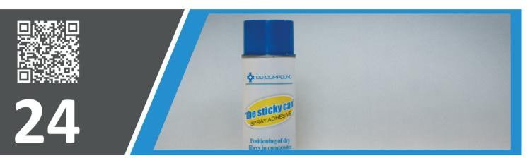
**The Sticky Can**® is a spray adhesive developed by DD-Compound. It is used to fix dry fibres in the mould for infusion setups. It sprays very fine and can be used for visual carbon parts. The Sticky Can does it transparent and will be embedded in the matrix after infusion. The tack is strong but it is still repositionable.
